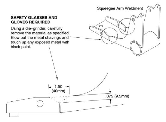
**NOTE:** After installing the replacement parts, cycle the ignition key on/off a couple of times to ensure proper clearance between the squeegee arm weldment and axle.
